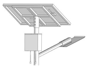
Screw fixed solar panel support to the poles, then connect lamp cable and solar panel cable with relative cable from battery box. Accessories: Screws: 4pcs
