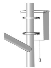
Screw fixed battery box to the pole. Accessories: Screws: 4pcs Nuts: 4pcs Gaskets: 4pcs Spring shim: 4pcs Hoops: 2pcs
